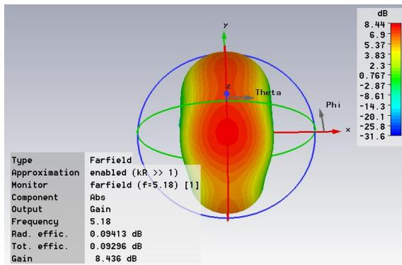
Fig. 7. The radiation pattern of the microstrip patch antenna at 5.18GHz
