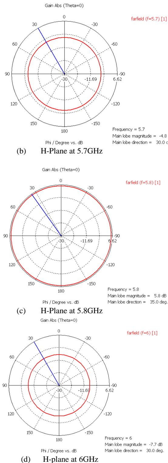
Fig. 10. Fairfield H-plane radiation patterns of proposed antenna at (a) 5.18GHz (b) 5.7GHz, (c) 5.8GHz, (d) 6GHz.
