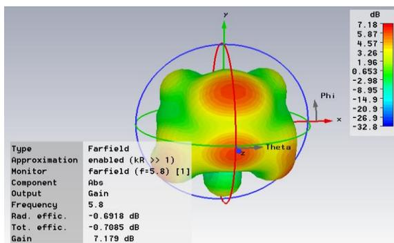
Fig. 8 The radiation pattern of the microstrip patch antenna at 5.8GHz
