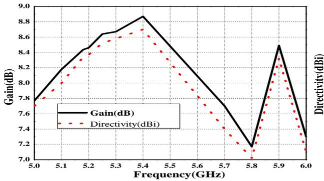
Fig. 6 Gain (dB)/Directivity (dBi) versus Frequency (GHz) of proposed antenna
