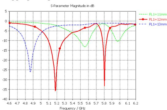
Fig. 4. Return losses from optimization of patch (PL1) of antenna
