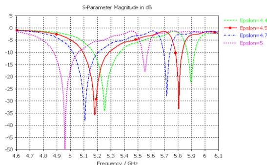
Fig. 5. Return losses from optimization of dielectric constant of the substrate
