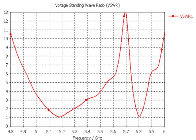
Fig. 11. Simulated VSWR of the proposed antenna.
