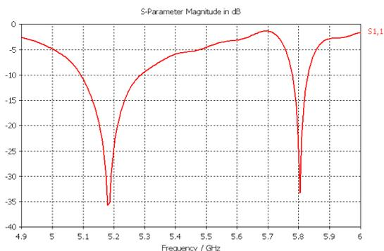
Fig. 3. Simulated return loss for the proposed dual band microstrip patch antenna at 5.18 GHz and 5.8 GHz.
